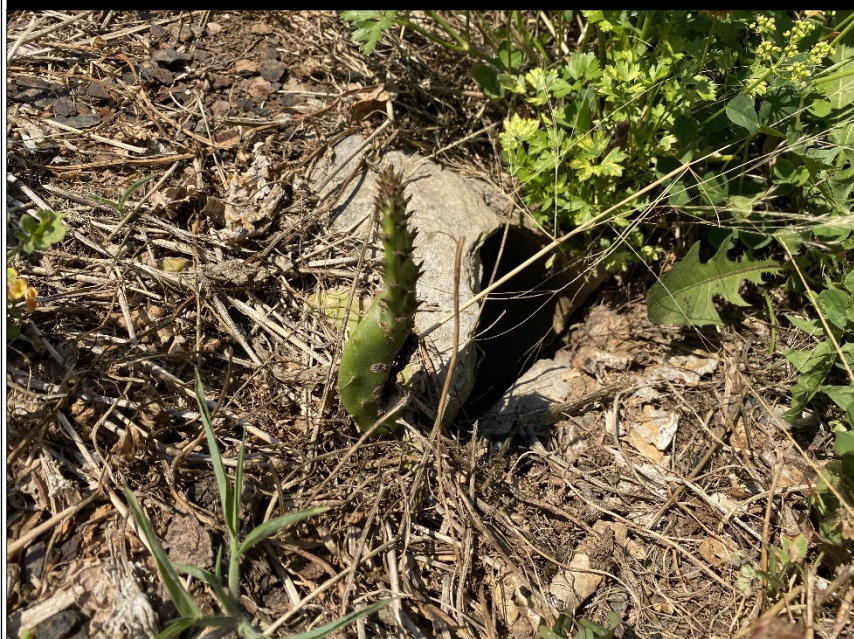
PHOTO 48: LOT L1 - SHOWING EXPOSED POTENTIAL ACM PIPE ADJACENT SHED
